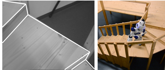
Fig. 1. Left: Camera image and projected staircase model based on the MCL pose estimate. The pose estimate is highly accurate as the model edges fit the edges in the camera image. Right: Nao climbs up a spiral staircase using our approach.
